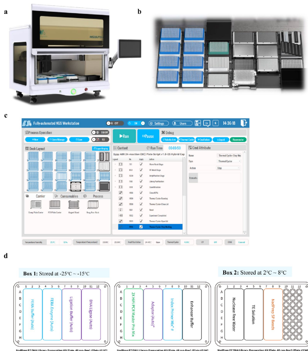
Fig. 1. Overview of the automated NGS workstation. (a) Front view of the automated workstation used in this study. (b) Top view of the configurable deck layout. (c) Screenshot of the software control interface. (d) Plate-based reagent format used for automated DNA library preparation.
