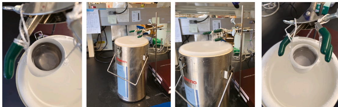
Figure 1. Setup of liquid nitrogen workstation for freezing mouse brain tissue
